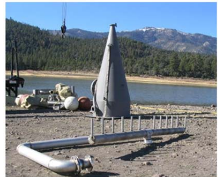
Figure 4-8. Speece Cone for in-lake installation and diffusers
